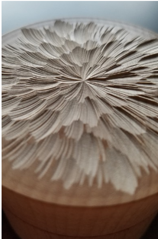
Sample box top texture #1, "Harmonic Power-Carving" (HPC) (Sugar Maple, 2.75" dia.)
