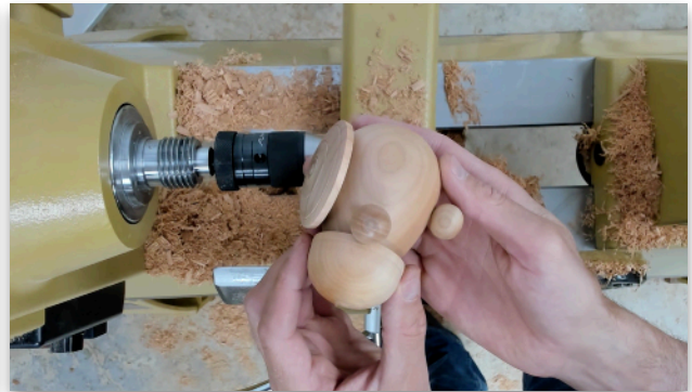
Photo 10 Drilling joinery holes completed. Dry fit.
